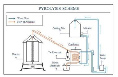
Figure 1. Pyrolysis Device Series Scheme
