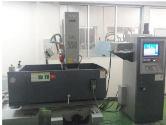
Gambar 1 Mesin *EDM sinking* Aristech LS-55
